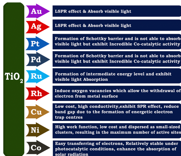
Fig. 5 Schematic representation of various noble metals used for improving the photocatalytic hydrogen evolution activity of TiO 2 .
