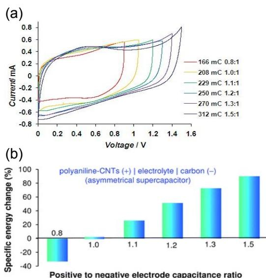
Figure 8. (a) CVs and (b) the specific energy of the cell of “polyaniline/carbon nanotubes | 1.0 M HCl | carbon” at the indicated positive to negative capacitance ratios. Reproduced from ref. <sup>137</sup> with permission from RSC Publishing, copyright 2010.
