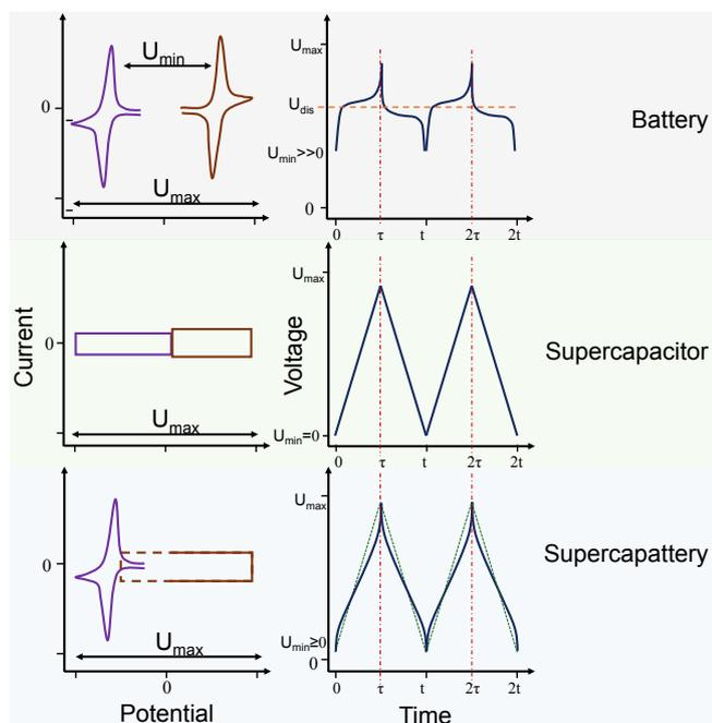
Figure 3. Illustration of CVs of electrodes and GCD profiles of two-electrode cells of battery, supercapacitor and supercapattery. (Redrawn from Ref. <sup>50</sup>)
