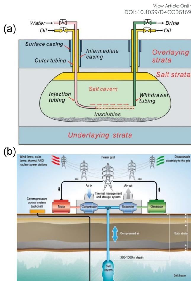
Figure 1. Schematic illustrations of (a) two well horizontal salt cavern construction, reproduced from ref. <sup>25</sup> with permission from Taylor & Francis, copyright 2020 and (b) compressed air energy storage in salt caverns, reproduced from ref. <sup>26</sup> with permission from Elsevier, copyright 2021.
