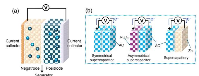
Figure 2. Schematic illustrations of (a) the structure of a generic EES device (cell) and (b) charging three different EES devices as indicated.
