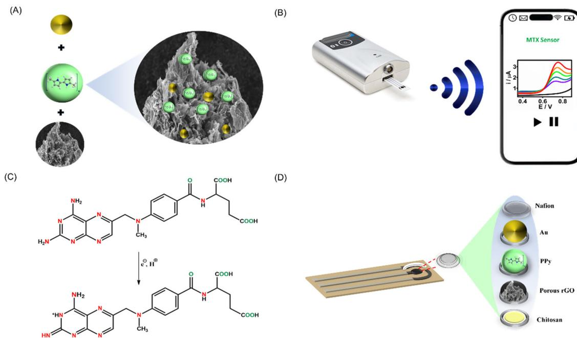
**Fig. 1** Diagrams showing the synthesis and sensing process. (A) The PrGO-PPy-Au nanocomposite. (B) Recording voltammograms of methotrexate using a bluetooth-enabled handheld potentiostat and a mobile device. (C) Electrochemical oxidation behaviour of methotrexate. (D) Diagram depicting the modified SPCE sensor's layered architecture incorporating a PrGO-PPy-Au composite within a chitosan matrix and protected by a Nafion layer.
