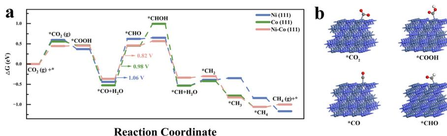
**Fig. 5** (a)  $\text{CO}_2$  hydro-methanation pathway on the Ni (111), Co (111) and Ni–Co (111) interface. (b) The optimized configurations of the key intermediates of Ni–Co (111). The blue, purple, grey, red and white spheres represent Ni, Co, C, O and H atoms, respectively.
