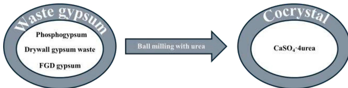
Figure 5. The process of using industrial by-product wastes to produce \text{CaSO}_4 \cdot 4\text{urea} (40,42)
