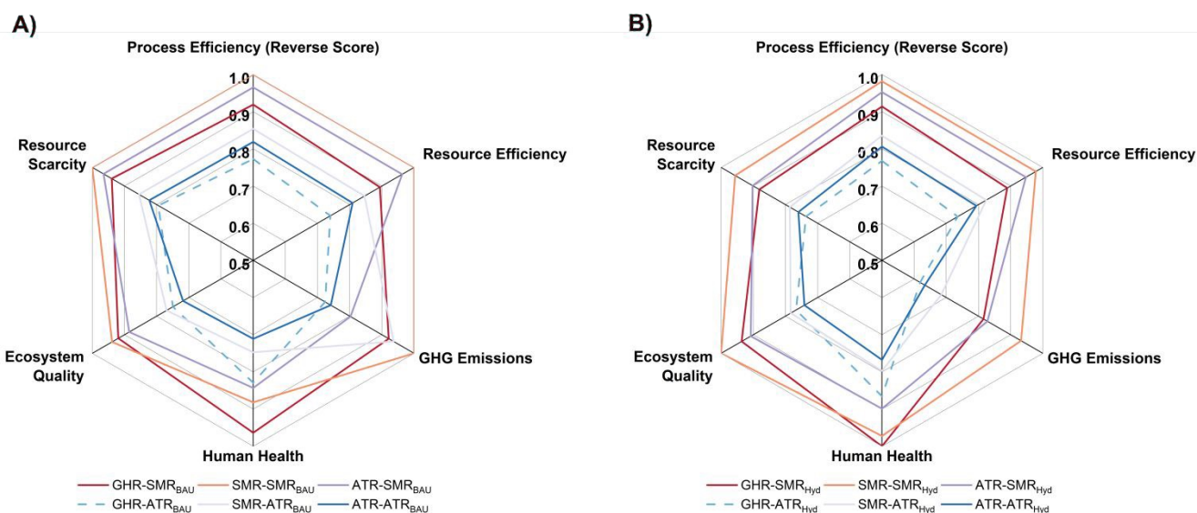
468 469 470 Fig. 6 Sustainability Analysis of A) BAU and B) IS integrated MeOH-NH 3 co-production 471 flowsheets. The blue dashed line [---] in both spider plots indicates the best-performing co- 472 production flowsheet, which meets all decision criteria. This flowsheet was chosen as it has the 473 smallest internal area and, thus, provides optimum results.
