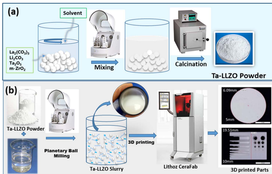
Fig. 4 (a) Synthetic scheme of LLZO powder and (b) fabrication process of 3D printed parts.
