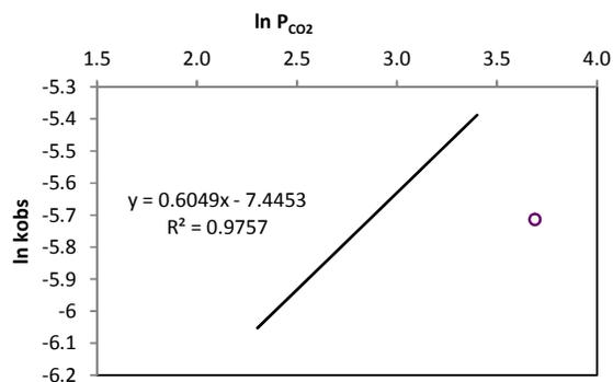
**Fig. 8** Styrene carbonate synthesis at four different CO<sub>2</sub> pressures (10-40 bar). Reaction conditions: T = 80 °C, **1** 0.2 mol %, TBAB 0.2 mol %.
