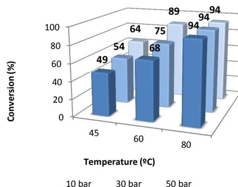
Fig. 4 Effect of CO<sub>2</sub> pressure and temperature on the coupling of 1,2-epoxyhexane and CO<sub>2</sub> using **1**/TBAB catalyst system. Reaction conditions: catalyst 0.2 mol%, TBAB 0.2 mol%, 18h. Reactions were run in duplicate.
