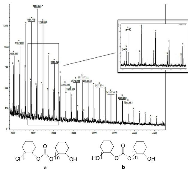
**Fig. 6** MALDI-TOF mass spectrum of polycarbonate from entry 4, Table 3
