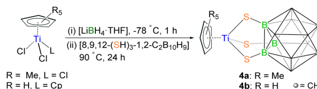
Scheme 3 Synthesis of 8,9,12-trithiol-o-carborane protected Ti-thiolate complexes 4a and 4b .
