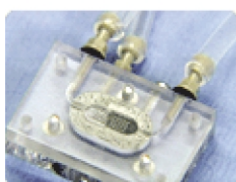
Fig. 4 (a) Schematic of scaffold and reactor housing. 41 (b) The silicon microfluidic chip in a polycarbonate housing [www.easternplastics.com].
