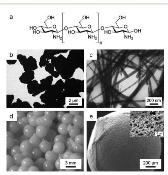
**Fig. 12** (a) Structure of chitosan. TEM images of samples of  $YBa_2Cu_4O_8$  synthesized using (b) acetate/tartrate and (c) chitosan. (d) Photograph and (e) SEM image of chitosan beads prepared by crosslinking with  $Ce^{3+}$  with (inset) SEM image of sponge-like structure formed after calcination of the beads. Images reproduced with permission from ref. 11 (b, c) and 109 (d, e).
