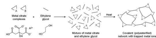
Fig. 6 Schematic of the Pechini method of making metal/organic gels.
