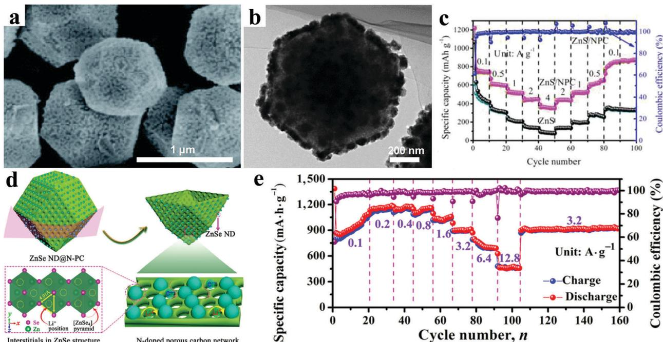
Fig. 13 (a) SEM image, and (b) TEM image of ZnS/NPC hybrid; (c) rate performances of ZnS/NPC and ZnS. Reproduced with permission.<sup>186</sup> Copyright 2017, Royal Society of Chemistry. (d) Schematic illustration for the construction of ZnSe ND@N-PC architecture; (e) rate capability at various current densities of ZnSe ND@N-PC composite electrodes. Reproduced with permission.<sup>191</sup> Copyright 2017, Tsinghua University Press and Springer.
