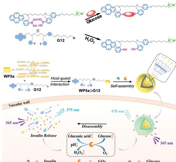
Fig. 15 Schematic illustration of the insulin delivery nanocarriers based on **WP5a** and **G12** with glucose-responsiveness. Reproduced with permission from ref. 102. Copyright 2018, Wiley Publishers.
