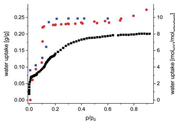
**Fig. 2** Gravimetric water adsorption isotherm collected at 298 K for Fe-MIL-59 (red dots), activated at 100 °C and  $10^{-2}$  mPa; water content obtained from Rietveld analyses (Table S1.1, ESI<sup>†</sup>) of PXRD data collected at different relative humidity values at 298 K (blue squares) and water uptake obtained from GCMC simulations (black squares).
