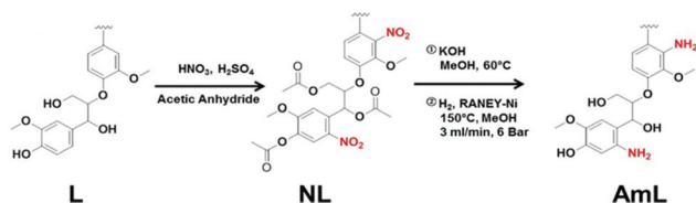
Fig. 2 Synthetic pathway for the conversion of alkali-lignin (L) into aminated lignin (AmL) via aromatic nitration.
