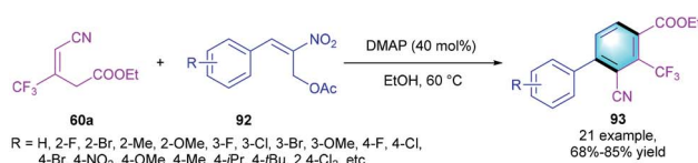
Scheme 24 DMAP-catalyzed [4 + 2] benzannulation to synthesize penta-substituted benzenes.
