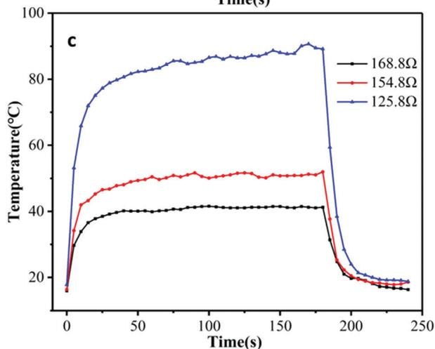
Fig. 4 (a) Temperature profiles of the GNP fabric at different  $V_{\text{GNP}}$ ; (b) temperature response of the GNP fabric over 5 cycles at  $V_{\text{GNP}} = 12$  V, each cycles is 4 min long; (c) temperature profiles of the GNP fabric operated at different biases.
