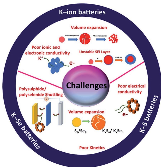
Fig. 3 Schematic of the challenges of potassium batteries.
