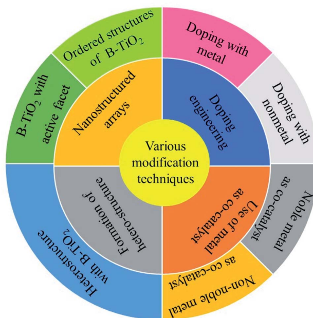
Scheme 2 Schematic diagram shows various modification techniques for B-TiO 2 to increase the hydrogen generation rate.
