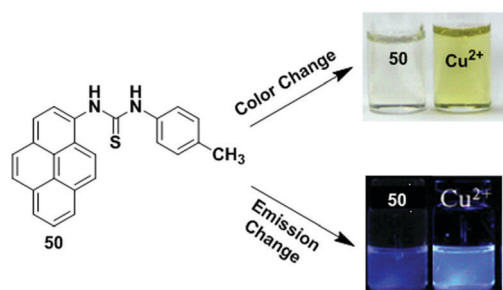
Fig. 44 The colour and fluorescence changes of chemosensor 50 upon addition of \text{Cu}^{2+} ions. Reproduced from ref. 119 with permission from the Elsevier, copyright 2010.
