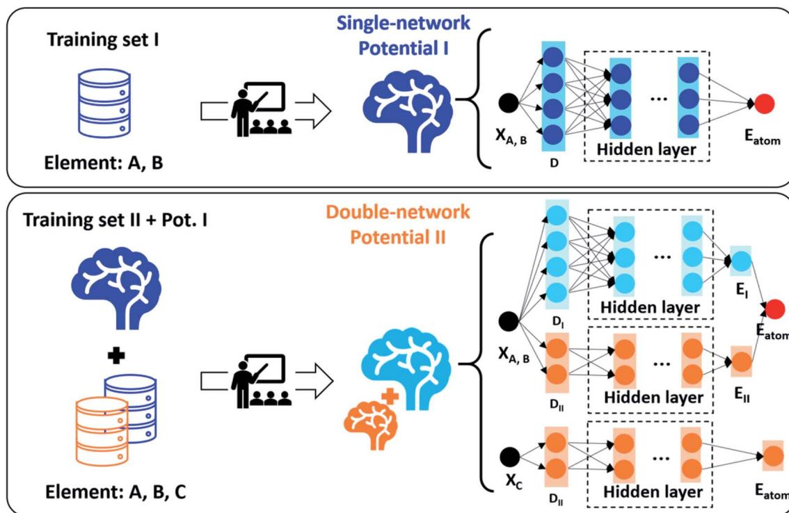
Fig. 8 A schematic illustration of the double-network framework.  $X$  represents the Cartesian coordinates of each atom.  $E_{atom}$  represents the atomic energy of each atom.  $D$  represents the structural descriptor. Reproduced from ref. 48 with permission from AIP Publishing, copyright 2021, licensed under a Creative Commons Attribution (CC BY) license.
