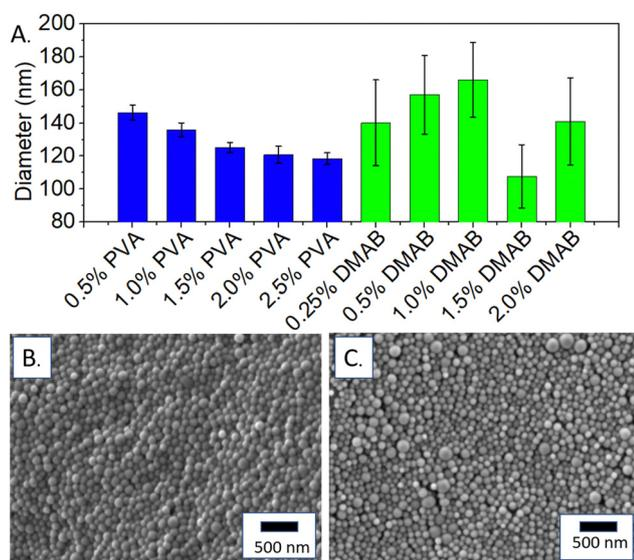
**Fig. 1** Size of PLGA nanoparticles made using PVA (blue) and DMAB (green) (mean  $\pm$  SD,  $n = 3$ ). Size decreases with increasing PVA concentration while particles prepared with DMAB have no clear trend and large error bars, indicating that the size of DMAB-PLGA particles is more variable. SEM image of PVA-PLGA NPs (B) and SEM image of DMAB-PLGA NPs (C).
