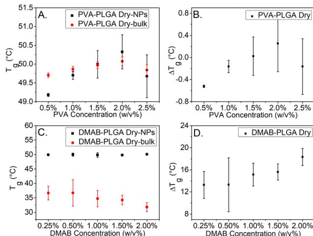
Fig. 7 Particle  $T_g$  and bulk  $T_g$  measured in dry condition for both PVA-PLGA (A) and DMAB-PLGA (C).  $\Delta T_g$  of PVA-PLGA (B) and DMAB-PLGA (D) in dry conditions (mean  $\pm$  SD,  $n = 3$ ).
