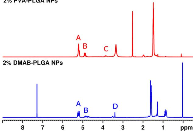
Fig. 3 NMR spectrums of 2% PVA-PLGA NPs in DMSO-d<sub>6</sub> (red) and 2% DMAB-PLGA NPs in CDCl<sub>3</sub> (blue).
