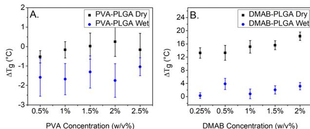
Fig. 10  $\Delta T_g$  of PLGA nanoparticles made with varying amounts of PVA (A) and DMAB (B) measured by mDSC either dry or in water.  $\Delta T_g$  represents the difference between nanoparticle  $T_g$  and bulk  $T_g$  (mean  $\pm$  SD,  $n = 3$ ).
