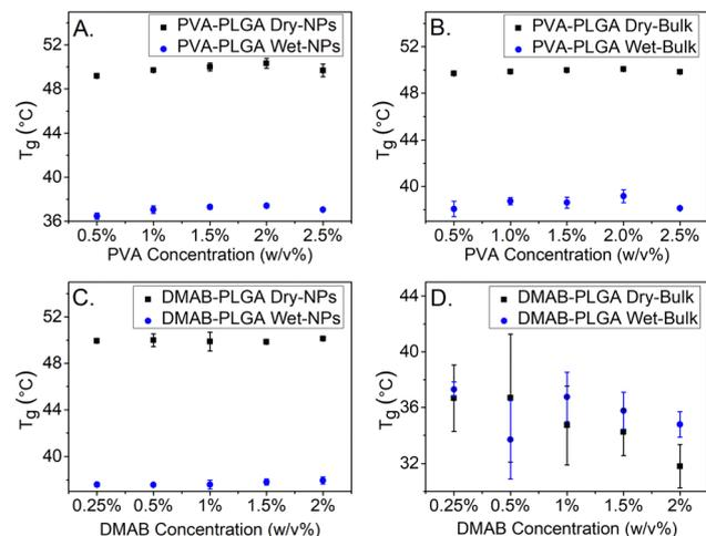
Fig. 8  $T_g$  of particles in dry and wet conditions vs. surfactant concentrations (A and C).  $T_g$  of bulk in dry and wet condition vs. surfactant concentrations (B and D) (mean  $\pm$  SD,  $n = 3$ ).
