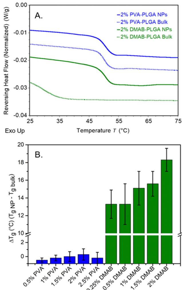
Fig. 9 Examples of mDSC plots (A) of PLGA nanoparticles (blue line) and bulk (blue dotted line) for 2% PVA-PLGA NPs (blue) and 2% DMAB-PLGA NPs (green), and (B)  $\Delta T_g$  of dry PLGA nanoparticles compared to the bulk  $T_g$  for nanoparticles made with varying amounts of PVA (blue) and DMAB (green).  $\Delta T_g$  of DMAB-PLGA nanoparticles is significantly higher than the  $\Delta T_g$  of PVA-PLGA nanoparticles (mean  $\pm$  SD,  $n = 3$ ). Curves shifted vertically for easier viewing.
