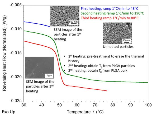
Fig. 5 DSC procedure and SEM images of PLGA nanoparticles. The blue curve represents the pre-treatment to erase thermal history while keeping the morphology of particles. Particle  $T_g$  was obtained from the second heating cycle (green curve). Bulk  $T_g$  was obtained from the third heating cycle (red curve). The SEM image of the sample after the third heating confirmed no particles existed in the last heating cycle. Curves shifted vertically for easier viewing.
