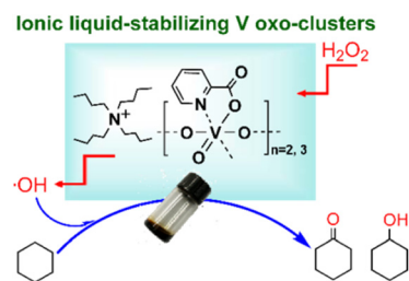
Fig. 4 IL-stabilized vanadium oxo-clusters catalyzing alkane oxidation. Adapted from ref. 63 with permission from Royal Society of Chemistry, copyright 2020.
