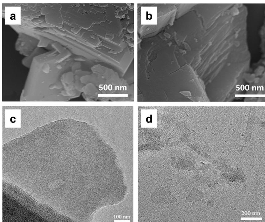
Fig. 5 SEM images of the 3D pillar-layered (a) Zn-MOF precursor and (b) Cu-MOF precursor and TEM images of the (c) 2D Zn-MOF nanosheet and (d) 2D Cu-MOF nanosheet.
