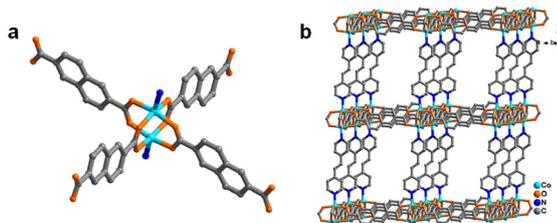
Fig. 1 (a) Coordinated structure of the Co-MOF with H<sub>2</sub>NDC as layer ligands; (b) three-dimensional pillared structure of the Co-MOF with bipyen as pillar ligands.
