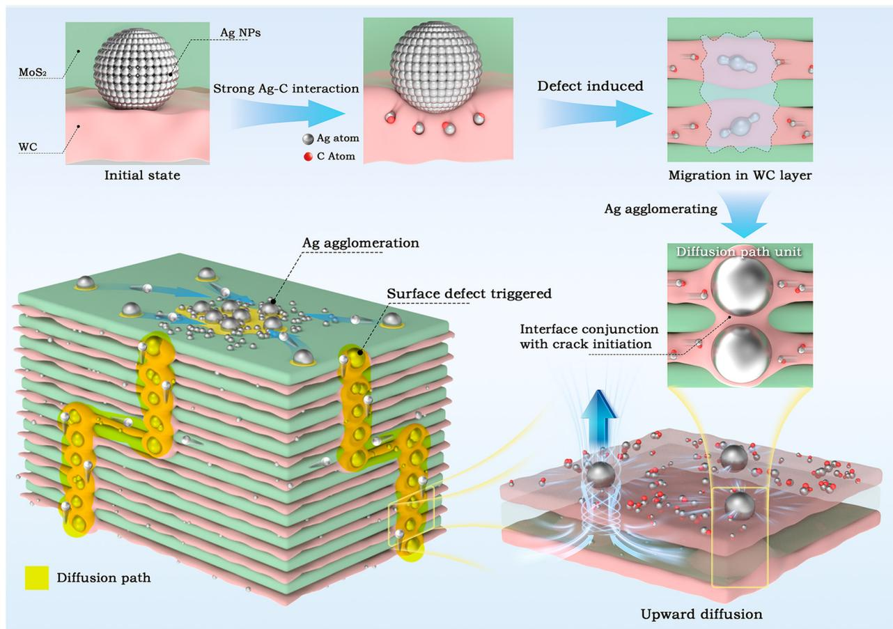
Fig. 7 Schematic of defect-dominated diffusion kinetics of Ag atoms within the sandwich-like MoS<sub>2</sub>/Ag/WC nanomultilayer film.
