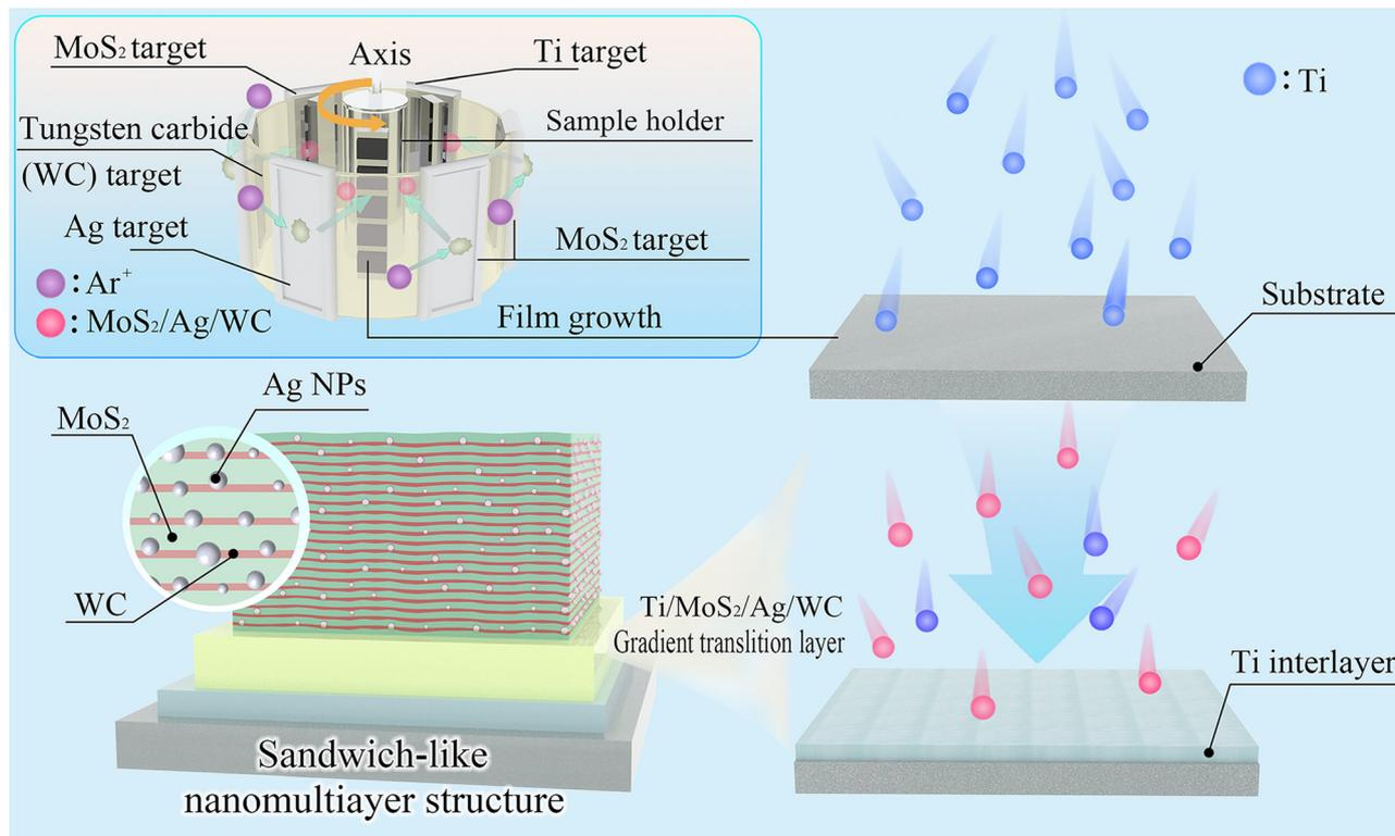
Fig. 1 Schematic illustrating the fabrication and structural design of the sandwich-like MoS<sub>2</sub>/Ag/WC nanomultilayer film.
