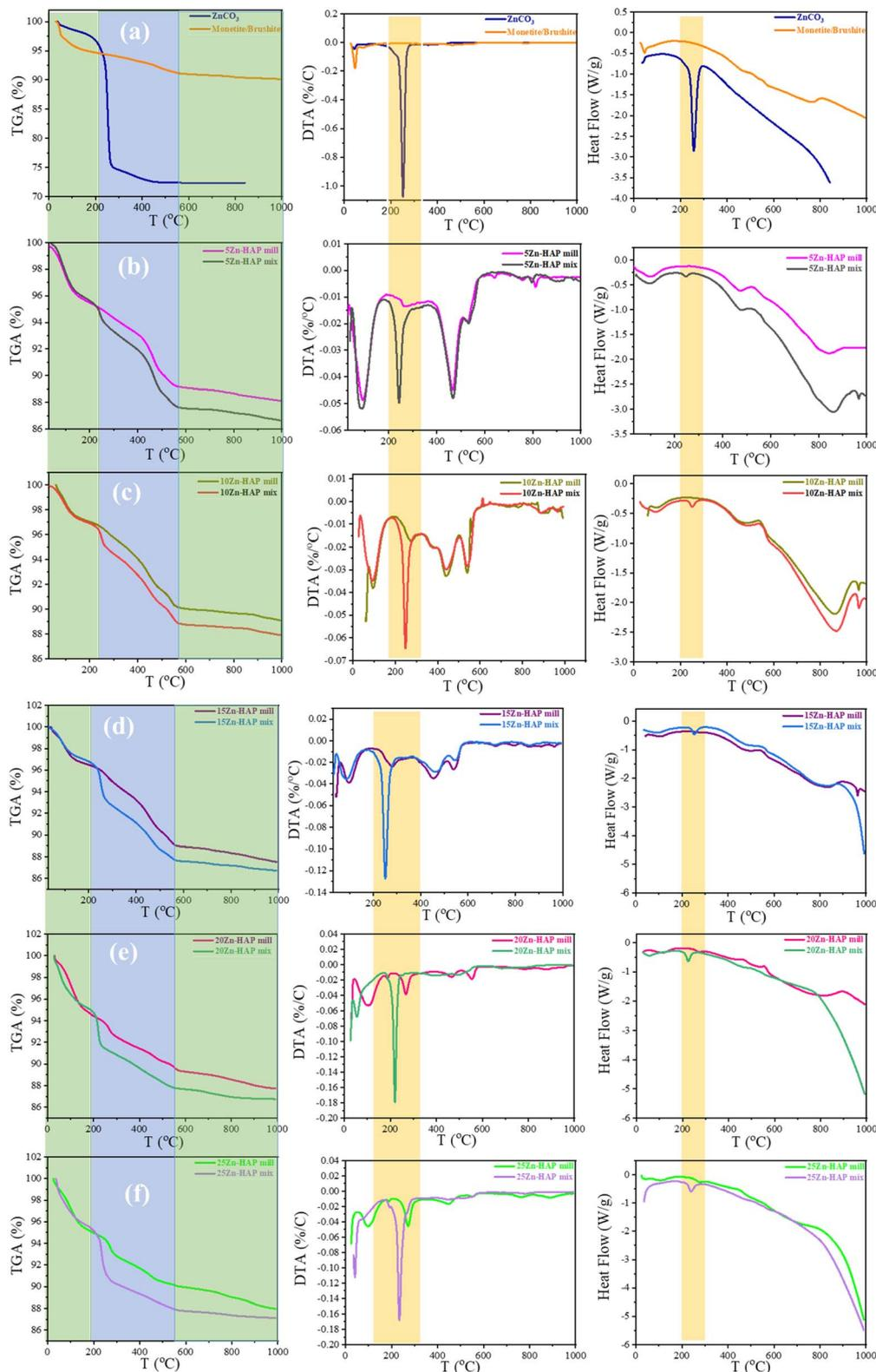
Fig. 5 TGA (left), DTA (middle), and DSC (right) for (a)  $\text{ZnCO}_3$  and monetite/brushite, (b) 5 Zn-HAP mill and 5 Zn-HAP mix, (c) 10 Zn-HAP mill and 10 Zn-HAP mix, (d) 15 Zn-HAP mill and 15 Zn-HAP mix, (e) 20 Zn-HAP mill and 20 Zn-HAP mix, and (f) 25 Zn-HAP mill and 25 Zn-HAP mix.
