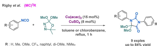
Scheme 4 Synthesis of hydantoin derivatives by Rigby et al.
