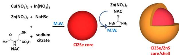
Scheme 1 Schematic representation of CIZSe and core/shell CIZSe/ZnS QDs synthesis.
