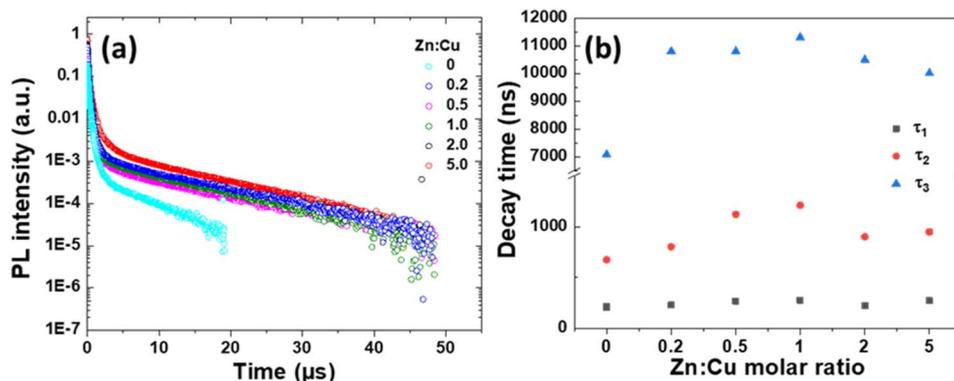
Fig. 2 (a) PL decay traces of CIZSe/ZnS QDs when varying the Zn : Cu molar ratio. PL decays were recorded at the PL maximum wavelength after excitation at 450 nm. (b) Evolution of  $\tau_1$ ,  $\tau_2$  and  $\tau_3$  decay times when varying the Zn : Cu molar ratio.
