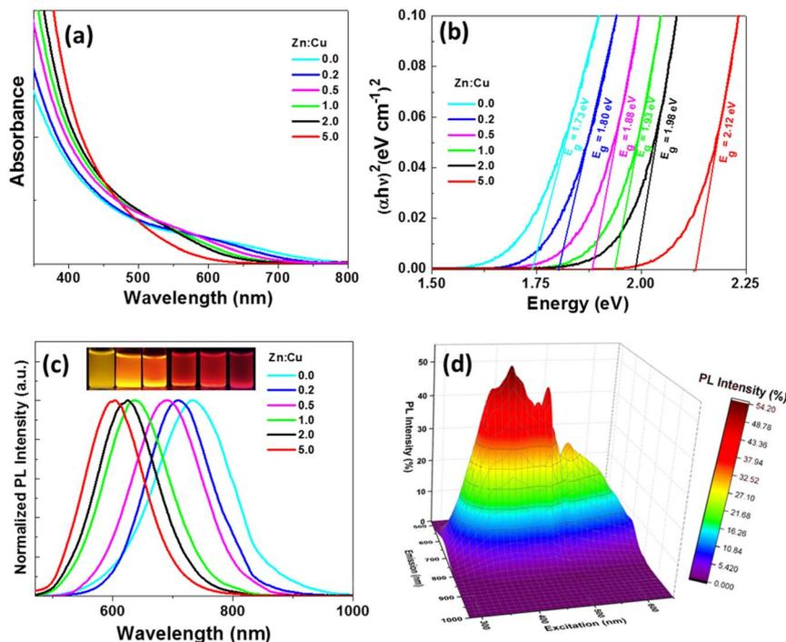
**Fig. 1** (a) UV-visible absorption spectra, (b) Tauc plots used for the determination of the optical bandgap, (c) PL emission spectra after excitation at 450 nm of CIZSe/ZnS QDs when varying the Zn : Cu ratio (the inset is a digital photograph of aqueous dispersions of QDs under UV illumination). (d) PL excitation-emission 3D map of CIZSe/ZnS QDs prepared with a Zn : Cu molar ratio of 0.5.
