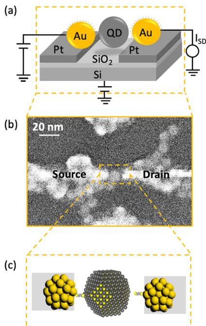
**Fig. 1** Resonant tunnelling transistor of a single PbS colloidal quantum dot. (a) Structure of a PbS QD RTT (schematic). (b) SEM image of ELGP HS-Au/Pt nanogap electrodes separated by a gap of  $\sim 9$  nm onto which PbS QDs ( $d \sim 8.1$  nm) have been one side-chemisorbed. (c) Simplified illustration of the magnified RTT with the top-view perspective. 1,2-ethanedithiol (EDT) is chemically anchored the PbS QD core to a spherical Au electrode.
