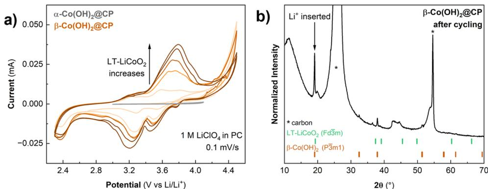
Fig. 5 (a) Cyclic voltammetry of  $\alpha$ -Co(OH)<sub>2</sub>@CP and  $\beta$ -Co(OH)<sub>2</sub>@CP in 1 M LiClO<sub>4</sub> in PC at 0.1 mV s<sup>-1</sup>. (b) XRD pattern of  $\beta$ -Co(OH)<sub>2</sub>@CP after cycling in 1 M LiClO<sub>4</sub> in PC showing partial transformation to spinel LT-LCO.
