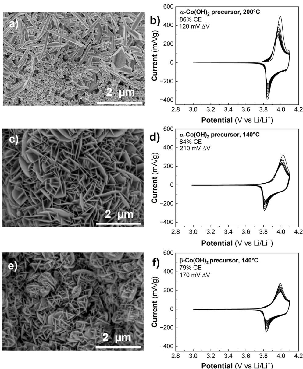
Fig. 7 Influence of hydrothermal temperature and Co(OH)<sub>2</sub> precursor phase on the synthesis of LCO@CP. SEM images and cyclic voltammograms of hydrothermal syntheses performed using (a and b)  $\alpha$ -Co(OH)<sub>2</sub>@CP at 200 °C, (c and d)  $\alpha$ -Co(OH)<sub>2</sub>@CP at 140 °C, and (e and f)  $\beta$ -Co(OH)<sub>2</sub>@CP at 140 °C. The vessel fill, LiOH concentration, and synthesis time were held constant at 11%, 4.4 M LiOH, and 120 h, respectively.
