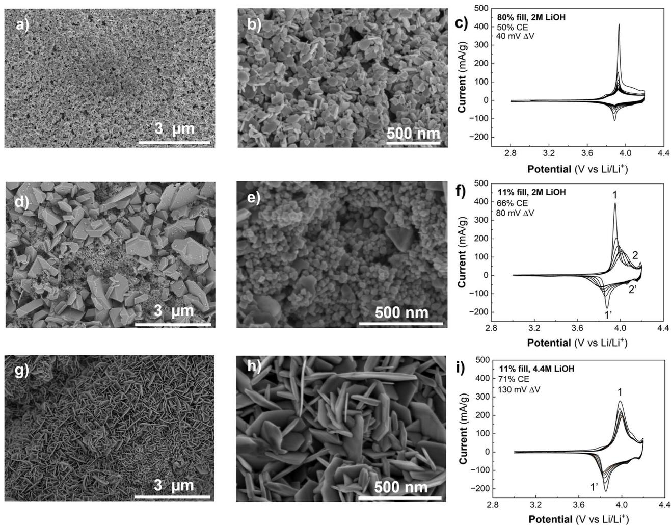
**Fig. 6** Influence of the hydrothermal synthesis pressure (% vessel fill) and LiOH concentration on the microstructure and performance of LCO@CP. SEM images and cyclic voltammograms of LCO@CP electrodes made using (a–c) 80% fill and 2 M LiOH, (d–f) 11% fill and 2 M LiOH, and (g–i) 11% fill and 4.4 M LiOH. The temperature and duration of hydrothermal synthesis were kept constant at 200 °C and 15 hours, respectively.
