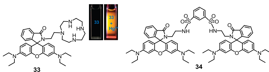
Figure 18. Molecular structures for receptors 33 [Inset: change in solution luminescence of 33 on binding to \text{Hg}^{2+} under Uv-light]; Structure of the chemosensor 34 . Reprinted with permission from ref 33. Copyright 2008 American Chemical Society.
