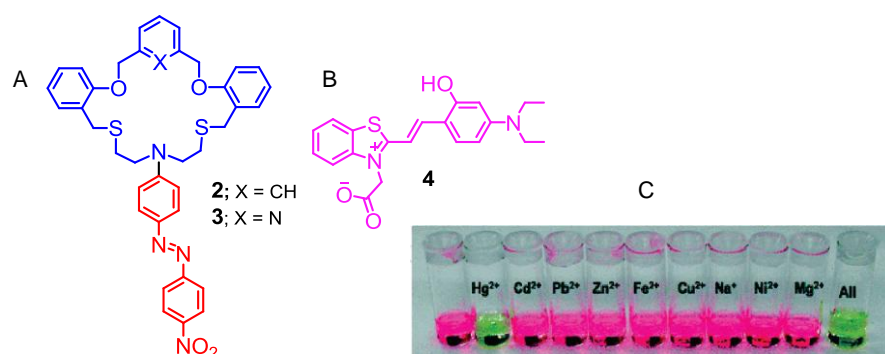
Figure 3. Molecular structure of chemosensors (A) 2 , 3 & (B) 4 ; (C) change in solution colour of 4 on binding to \text{Hg}(\text{II}) in 1:10 EtOH/ \text{H}_2\text{O} (pH 7, HEPES buffer). Reprinted with permission from ref 14. Copyright 2006 American Chemical Society.
