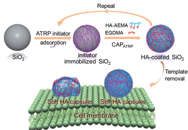
Scheme 1 Illustration of HA capsule formation and their cell surface binding behavior. Capsules are prepared via CAP ATRP using SiO 2 particles as templates, which includes ATRP initiator adsorption, ATRP-promoted HA film growth, and template removal.
