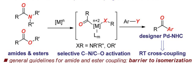
Fig. 1 (A) Cross-coupling of carboxylic acid derivatives. (B) The first general coupling of amides and esters at room temperature enabled by designer Pd–NHC catalysis (this work).
