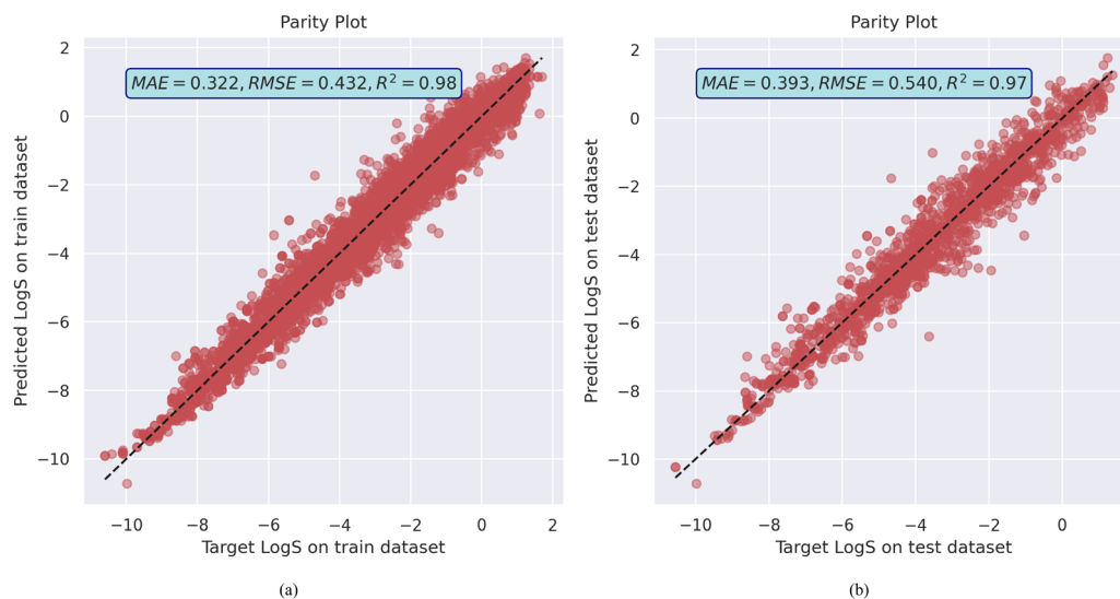
Fig. 1 MolGAT model training and validation performance on AqSolDB (a) the parity plot of predicted against target aqueous solubility values, and (b) the model train and test losses.
