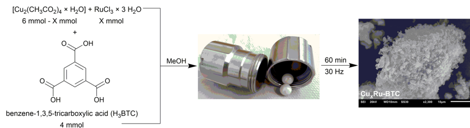
Fig. 1 Schematic representation of the synthesis of the mixed-metal \text{Cu}_x\text{Ru} -BTC MOFs.
