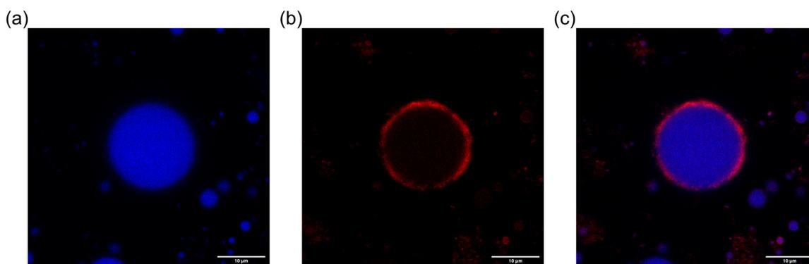
Fig. 4 Confocal laser scanning microscopy (CLSM) images of the WNIPU latex stabilized with CNC-RB at an  $m_p$  of  $8 \text{ mg mL}^{-1}$ . (a) Fluorescence detected under 405 nm excitation (WNIPU), (b) fluorescence detected under 561 nm excitation (CNC-RB), and (c) merged image of both channels. Scale bar:  $10 \mu\text{m}$ .
