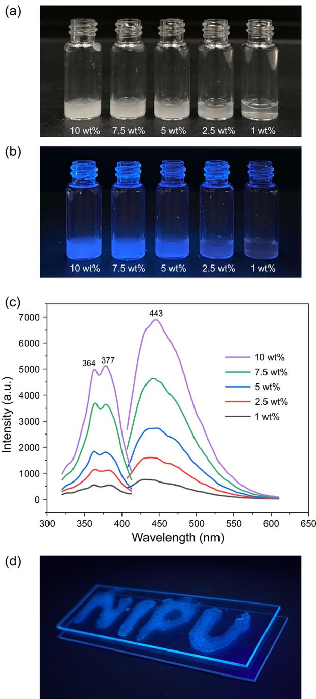
**Fig. 7** Photographs and fluorescence spectra of the aqueous WNIPU latex suspensions with varying solid contents. (a) Photographs taken under natural light, (b) photographs taken under UV irradiation ( $\lambda = 365$  nm), and (c) excitation and emission spectra recorded with aqueous suspensions. (d) Photograph of the letters "NIPU" written on a glass slide using the aqueous WNIPU latex suspension as ink, taken under 365 nm UV light (letters were written on the top glass slide).
