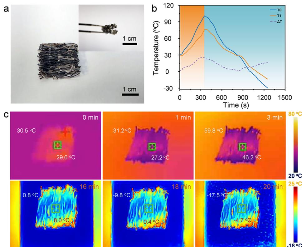
Fig. 5 Shape stability and thermal insulation tests of GO/SF@TPU-PEG fabric. (a) The pictures of GAF-PW after the shape stability test. (b) The temperature–time curve for the hot plate ( $T_0$ ), sample surface ( $T_1$ ) and temperature difference ( $\Delta T$ ) between  $T_0$  and  $T_1$ . (c) Thermal images of the fabric surface corresponding to the warming and cooling process.
