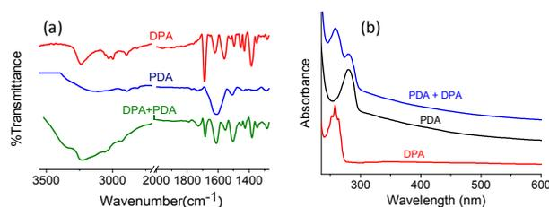
**Fig. 2.** (a) FT-IR transmittance spectra and (b) UV-Vis absorbance spectra for DPA, PDA and PDA co-assembled with DPA (condition 2).
