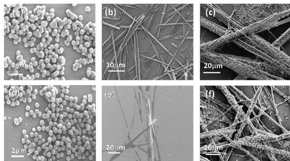
**Fig. 3.** Representative HR-SEM micrographs of the PDA spheres, DPA nanotubes and the co-assembled structures (condition 2) on a titanium surface before (a,b,c) and after (d,e,f) washing with water.
