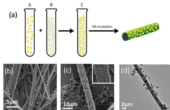
**Fig. 1.** (a) The scheme illustrates the co-assembly processes under condition 2 (Table 1); (A) PDA spheres in water (1mg/mL), (B) DPA in HFP (100mg/mL) and (C) PDA (1mg/ml): DPA (5mg/ml) in water (not to scale). (b) and (c) HR-SEM micrographs of the co-assembled structures under condition 1 and 2 respectively, (d) TEM micrograph of the co-assembled structures (condition 2) after 18h of incubation.
