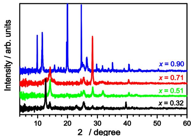
**Fig. 1** XRD patterns of  $(\text{MAI})_x(\text{PbI}_2)_{1-x}/\text{TiO}_2/\text{glass}$  samples as a function of the initial mole fraction  $x$  of MAI. The materials were deposited by a single-step deposition process from DMF. Black, green, red and blue lines are the XRD patterns for  $x = 0.32$ , 0.51, 0.71 and 0.90, respectively.
