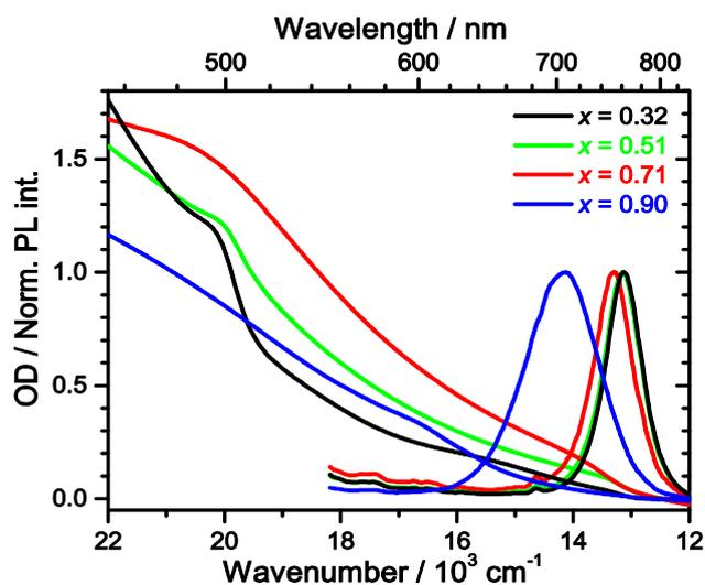
**Fig. 2** Steady-state absorption (left) and photoluminescence spectra (right) of  $(\text{MAI})_x(\text{PbI}_2)_{1-x}/\text{TiO}_2/\text{glass}$  prepared using different initial mole fractions  $x$  of MAI. Black: 0.32, green: 0.51, red: 0.71, blue: 0.90. For the sake of an easier comparison, absorption spectra are set to Zero at 840 nm. Photoluminescence spectra are normalized to their peak amplitude.
