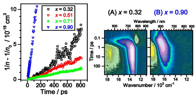
Broadband transient absorption spectroscopy reveals an increased carrier recombination rate constant of low-dimensional perovskites.
