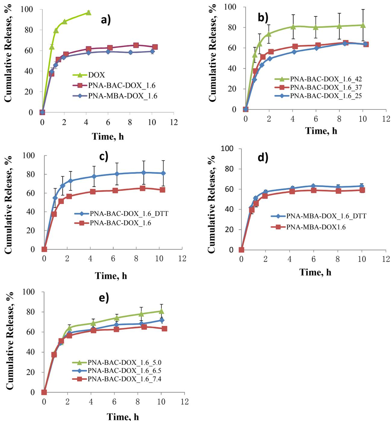
**Figure 4.** *In vitro* DOX cumulative release in PBS buffer from a) free DOX, PNA-MBA-DOX<sub>1.6</sub> and PNA-BAC-DOX<sub>1.6</sub> NGs at 37 °C, b) PNA-BAC-DOX<sub>1.6</sub> NGs at different temperatures (25, 37 and 42 °C), c) PNA-BAC-DOX<sub>1.6</sub> NGs and d) PNA-MBA-DOX<sub>1.6</sub> in the presence and absence of DTT (4.0 mM) at 37 °C, e) PNA-BAC-DOX<sub>1.6</sub> at different pH values (7.4, 6.5 and 5.0).
