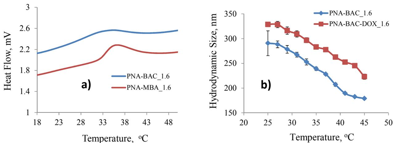
**Figure 3.** a) DSC curves of PNA-MBA\_1.6 and PNA-BAC\_1.6 samples; b) Hydrodynamic size of the PNA-BAC\_1.6 and PNA-BAC-DOX\_1.6 NGs in UP water as a function of temperature.
