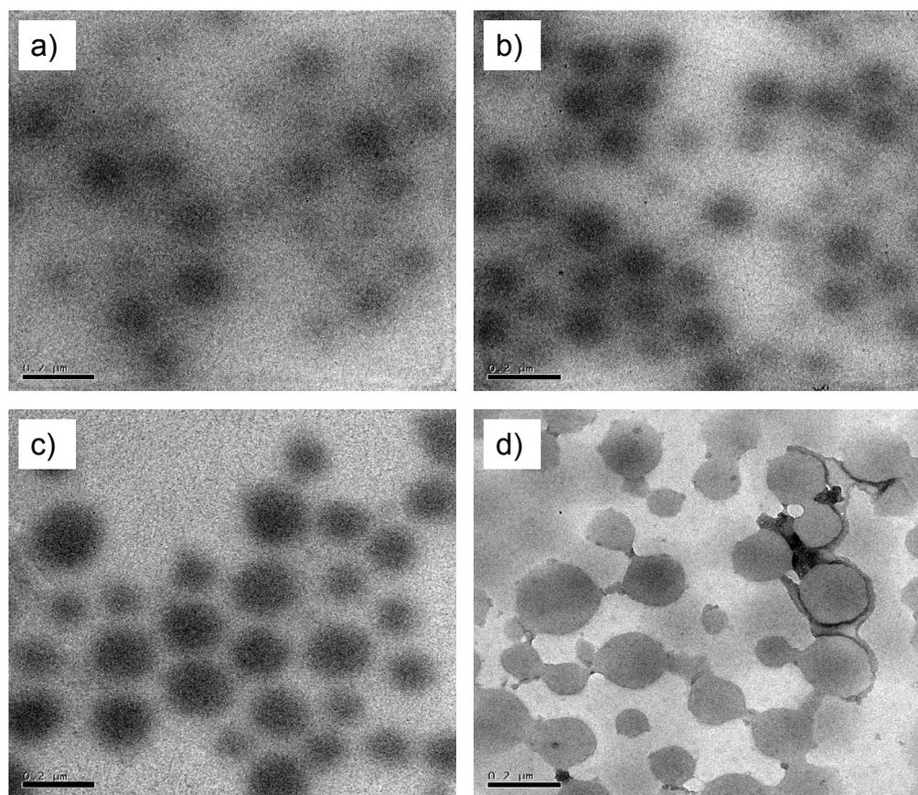
**Figure 2.** Transmission electron microscope (TEM) images of the PNA-BAC\_1.6 NGs in ultrapure water in the absence (a, b) and presence (c, d) of 4.0 mM DTT for a period of 0.5 h (a, c) and 10 h (b, d).
