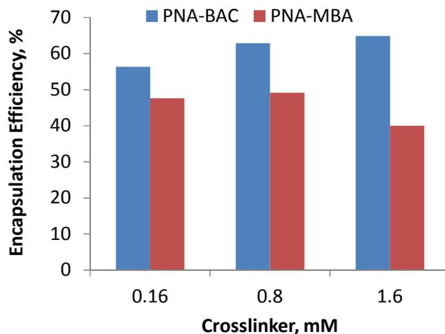
**Figure 1.** The effect of crosslinker concentration on DOX encapsulation efficiency (EE) of PNA-MBA and PNA-BAC NGs.
