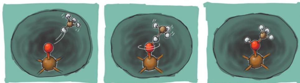
**Scheme 1** Proposed reaction mechanism of methane hydroxylation by  $[\text{FeO}]^{2+}$ -exchanged zeolites via a homolytic H-atom abstraction leading to the formation of a methyl radical and a subsequent methanol molecule. Adapted with permission from ref. 90. Copyright 2016 American Chemical Society.
