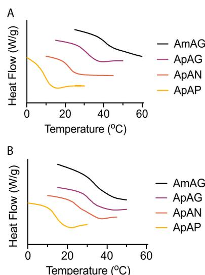
Figure 5. Differential scanning calorimetry of the (A) tetrathiol and, (B) trithiol cross-linked networks
