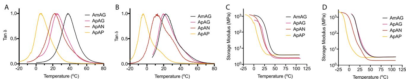
**Figure 6.** Thermal and mechanical properties of sequence defined networks (60 min. UV-cure). (A–D) Dynamic mechanical analysis of cross-linked networks. The  $\tan \delta$  curves of networks cross-linked with (A) tetrathiol and (B) trithiol. Plots of storage modulus (log scale) as a function of temperature for (C) tetrathiol cross-linked networks and (D) trithiol cross-linked networks.
