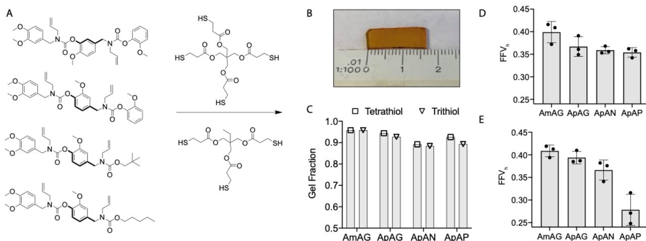
**Figure 4.** (A) Macromer cross-linking via a photo-initiated thiol-ene reaction with a tetrathiol and trithiol. (B) Image of crosslinked film (C) Gel fraction for each of the crosslinked networks after 60 minutes of irradiation. Fractional free volume of static holes ( $FFV_n$ ) of macromers crosslinked with the (D) tetrathiol, and (E) trithiol cross-linker.
