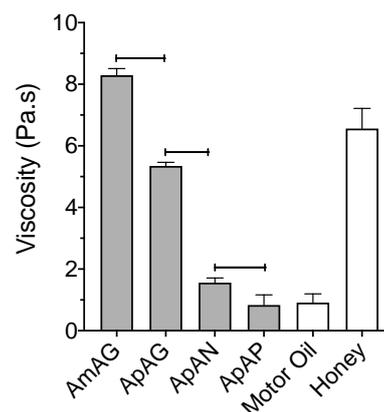
**Figure 3.** Viscosity measurements made with a parallel plate rheometer at a temperature of 45 °C and a constant shear rate of  $0.1 \text{ s}^{-1}$ . \*\*\*, p-value < 0.0001, \*, p-value < 0.05
