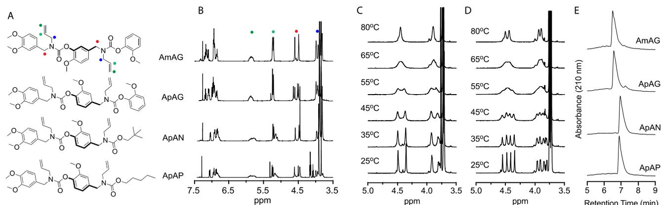
**Figure 2.** (A) Chemical structure of macromers evaluated in this study; (B)  $^1\text{H}$  NMR spectra of macromers; VT NMR of (C) AmAG and (D) ApAG; (E) Retention time of the macromers on a C4 reverse-phase column
