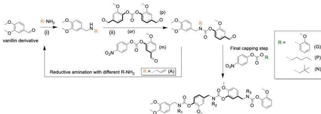
**Figure 1.** General synthesis scheme for sequence-defined polyurethane macromers. (i) MeOH, NaBH<sub>4</sub>, room temperature, (ii) triethylamine, CH<sub>3</sub>CN, 50 °C. (A) – allyl, (G) – guaiacol, (P) – pentyl, (N) – neopentyl.
