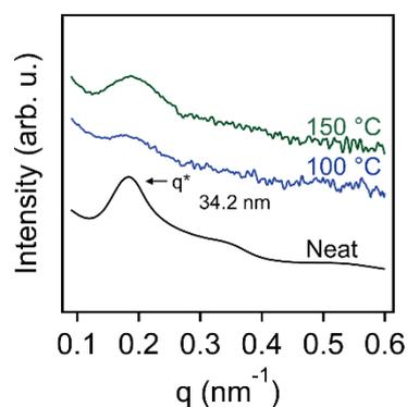
Figure 3. SAXS results for neat SBS in comparison to samples sulfonated at 100 °C for 60 min and 150 °C for 20 min, respectively.
