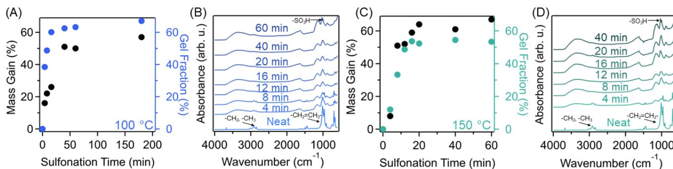
Figure 2. (A) Mass gain and gel fraction and (B) FTIR spectra of SBS reacted at 100  $^{\circ}\text{C}$  as a function of reaction time. (C) Mass gain and gel fraction and (D) FTIR spectra of SBS reacted at 150  $^{\circ}\text{C}$  as a function of reaction time.
