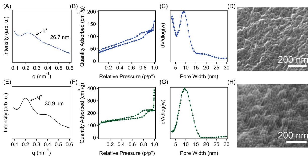
Figure 6. (A) SAXS pattern, (B) nitrogen physisorption isotherm, (C) NLDFT calculated pore size distribution, and (D) SEM image of the SBS100. (E) SAXS pattern, (F) nitrogen physisorption isotherm, (G) NLDFT calculated pore size distribution and (H) SEM image of the SBS150.
