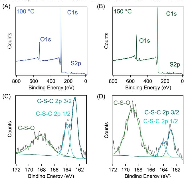
Figure 7. (A,B) XPS survey scans for SBS100 and SBS 150, respectively. (C,D) Corresponding high resolution S2p scans of SBS100 and SBS150, respectively.
