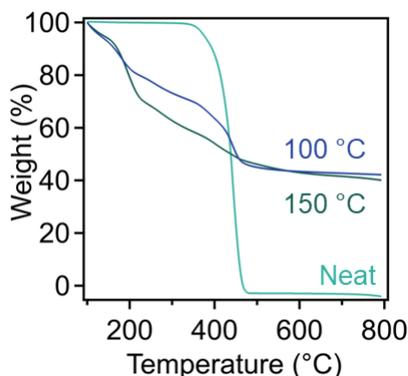
Figure 4. TGA thermogram of neat SBS, SBS sulfonated at 100 °C for 60 min, and SBS sulfonated at 150 °C for 20 min.
