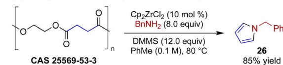
Scheme 2 Applications to polyester depolymerization. ( a Reported values are based on the theoretical amount of repeating monomer unit).
