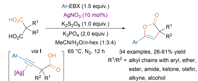
Scheme 34 Ag-catalyzed monodecarboxylative alkynylation–lactonization of malonic acid derivatives.
