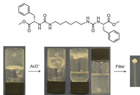
Fig. 41 Structure of a urea-based gelator used to control API crystallisation and photographs of the growth of a crystal of carbamazepine within the gel, and the use of acetate anions to disassemble the gel and allow recovery of the crystal. Figure reproduced from ref. 331 with permission of Springer Nature, © 2010.
