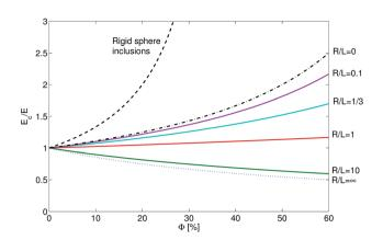
**Fig. 4** The stiffness of soft composites. Young's modulus of composites of droplets embedded in linear-elastic solids,  $E_c$  as a function of liquid content. The dotted curve shows Eshelby's prediction without surface tension. The dash-dotted curve shows the surface-tension dominated limit,  $R/L \ll 1$ . The dashed curve show Eshelby's prediction for rigid spheres embedded in an elastic solid.
