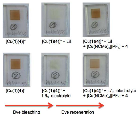
Fig. 8 Photographs of electrodes used for the dye bleaching and regeneration tests.
