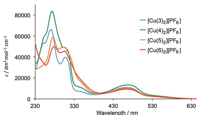
Fig. 2 Solution (CH<sub>2</sub>Cl<sub>2</sub>) absorption spectra of complexes [Cu(L<sub>ancillary</sub>)<sub>2</sub>][PF<sub>6</sub>] with L<sub>ancillary</sub> = **3–6** (5 × 10<sup>-5</sup> mol dm<sup>-3</sup>).
