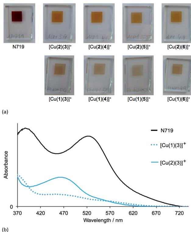
**Fig. 4** (a) Photographs of the electrodes. (b) Solid-state absorption spectra of  $\text{TiO}_2$  functionalized with  $[\text{Cu}(1)(3)]^+$ ,  $[\text{Cu}(2)(3)]^+$  or N719. Spectra were background-corrected by subtraction of the absorption spectrum of a blank electrode, then normalized for zero absorption at  $800 \text{ nm}$ .
