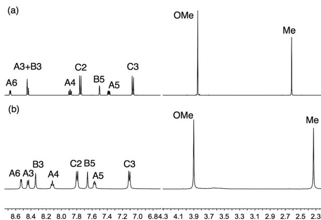
Fig. 1 500 MHz NMR spectra of (a) ligand **5** in CD<sub>3</sub>CN, and (b) [Cu(**5**)<sub>2</sub>][PF<sub>6</sub>] in CD<sub>2</sub>Cl<sub>2</sub> (≈ 295 K). For atom labelling, see Scheme 2. A common solvent could not be used for ligand and complex.
