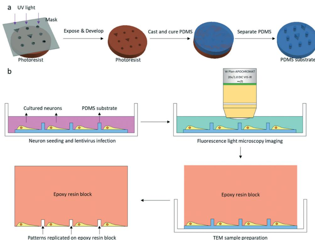
**Fig. 1** Schematic of PDMS substrate fabrication, fluorescence light microscopy imaging, and transmission electron microscopy (TEM) sample preparation. (a) The conventional soft lithography method is used for PDMS substrate fabrication, and the patterns are custom-designed for FLM and EM correlation. (b) FLM imaging and TEM sample preparation. After FLM imaging, the TEM sample is prepared in the dish. Patterns designed on PDMS are replicated on the epoxy resin block.
