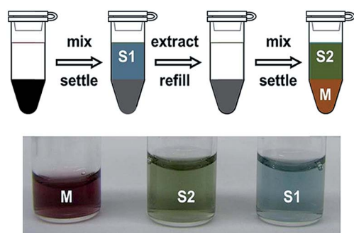
Fig. 6 (Top) Schematic of band gap fractionation of a SWCNT sample by sequential ATPE separations at successively reduced oxidant concentrations. (Bottom) Photographs of separated fractions isolated from a small diameter SWCNT population. Adapted with permission from Gui et al. , Nano Lett. , 2015, 15, 1642–1646. Copyright 2015 American Chemical Society.
